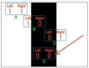
Finally, we need to check for case D - both sensors are 0 so we are on the track, and just need to go forwards.
