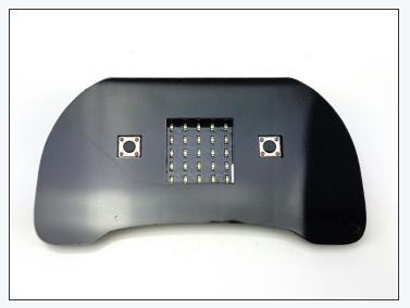
Peel the packing off of the 4 sticky squares, and stick the micro:bit onto the controller plate as shown in the picture.
